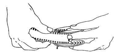
FIGURE 4-4. WINDING ONTO REEL
