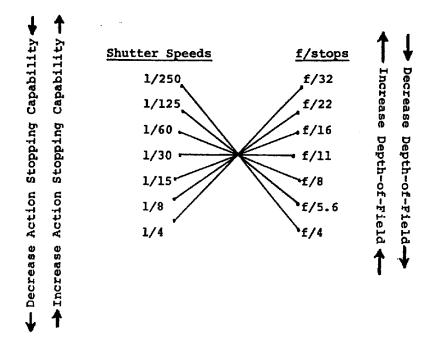
FIGURE 1-8. DEPTH OF FIELD VS ACTION STOPPING CAPABILITY
